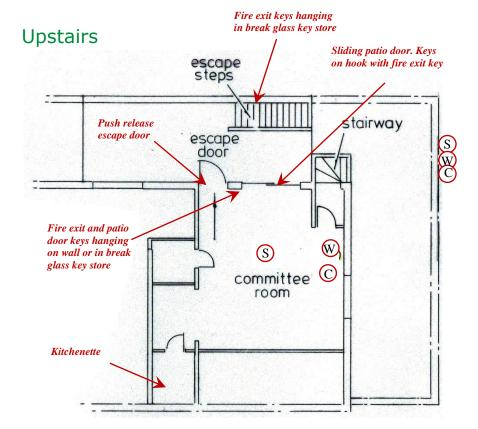
Smoke alarm Water extinguisher CO<sub>2</sub> extinguisher
