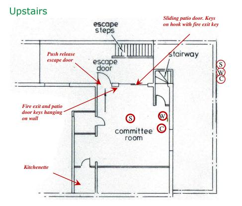
Smoke alarm Water extinguisher CO<sub>2</sub> extinguisher
